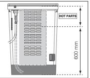
**Important:** make sure the supply pressure conforms with the values shown in the table entitled "Caracteristics of the burners and nozzles". When the cooker is installed between cabinets (recessed), the gas connection must be effected by an approved flexible hose with bayonet fitting (BS 669 Current Edition). The gas inlet for the cookers is a threaded G 1/2 gas female fitting.
